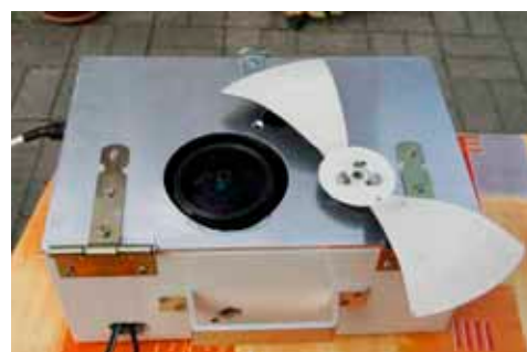
All-Sky camera equipment at station Wilderen, Belgium operated by Jean-Marie Biets. Note the 2-blade rotating shutter in front of the lens.
